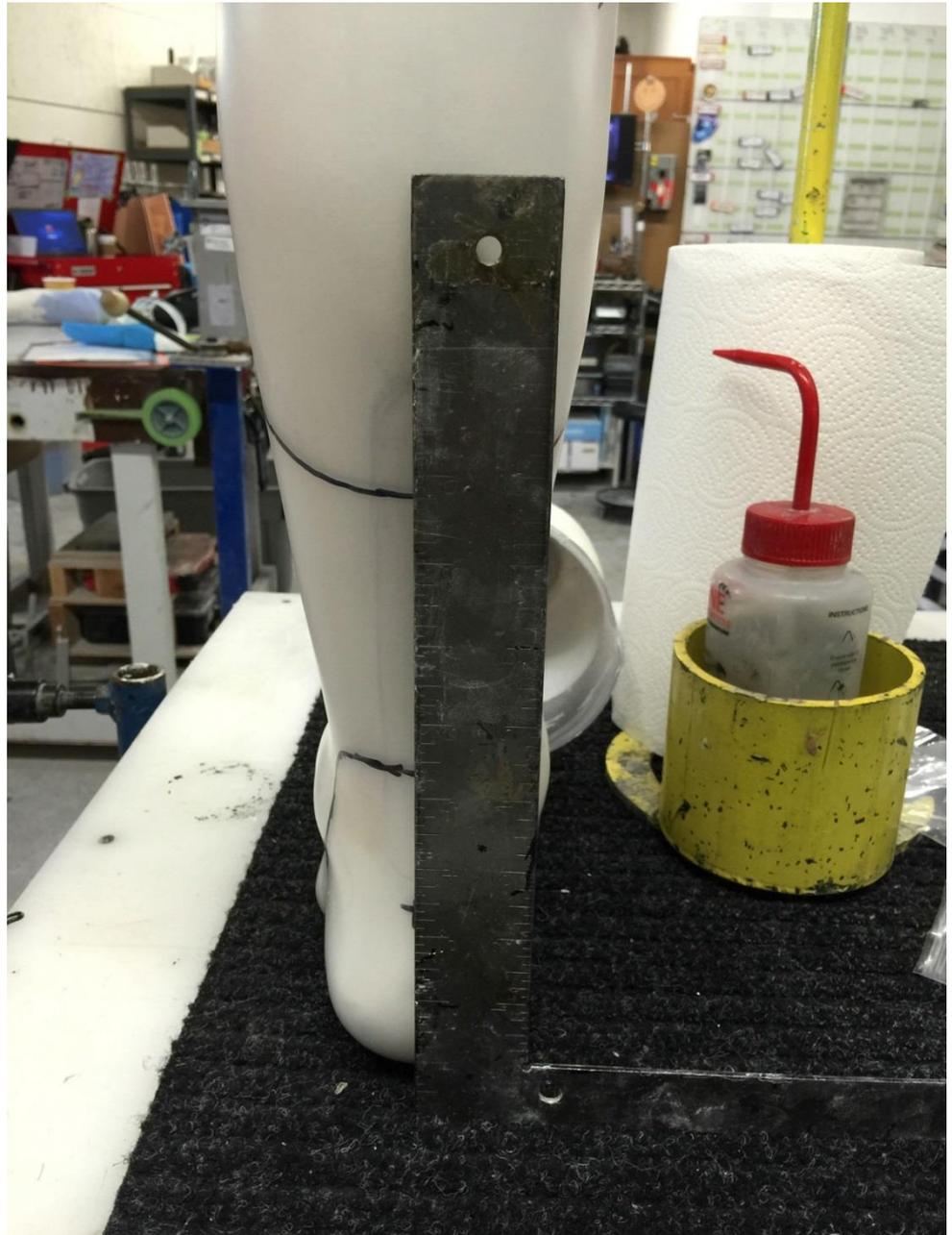
This reference mark is the ideal placement for the spring. In the event this mark is noticeably off center of the calf it is ok to alter it within a few degrees for aesthetics.
