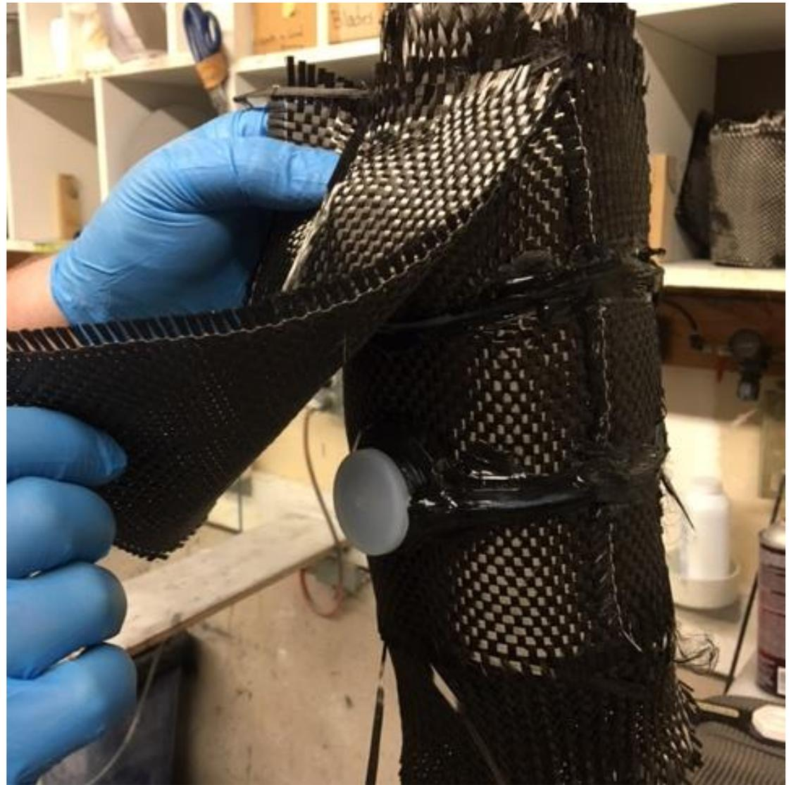
Form 12K 0/90 carbon tape over the BOA Closure System. Make sure it “locks” the system in well, as this will help hold it in position when laminating with resin.
