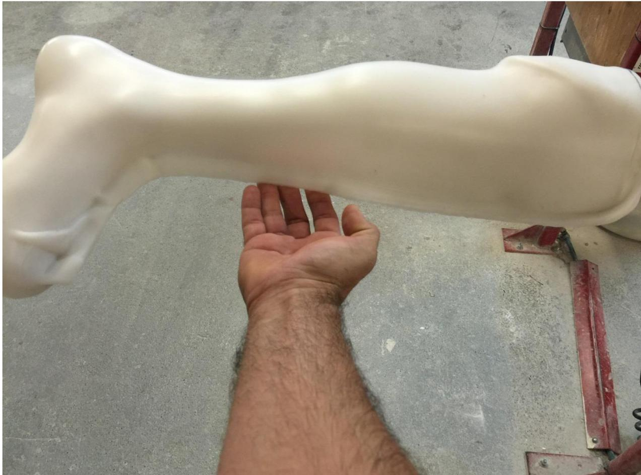
Keep the plastic join/seam as clean and straight across the shin section as possible. Trim away all excess plastic. Using grinding and buffing equipment smooth the plastic join/seam on the shin section focusing on the area within the trim lines.
