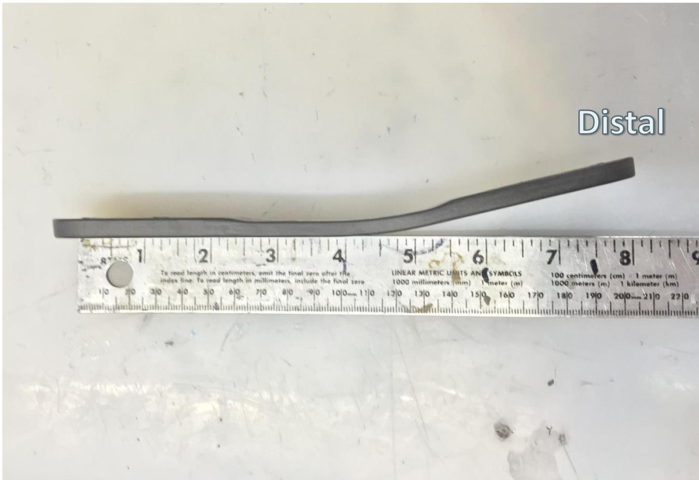
**The PDE spring is not symmetrical. The bend is closer to the distal end of the spring. Shown here the distal location of the spring is to the right side.**
