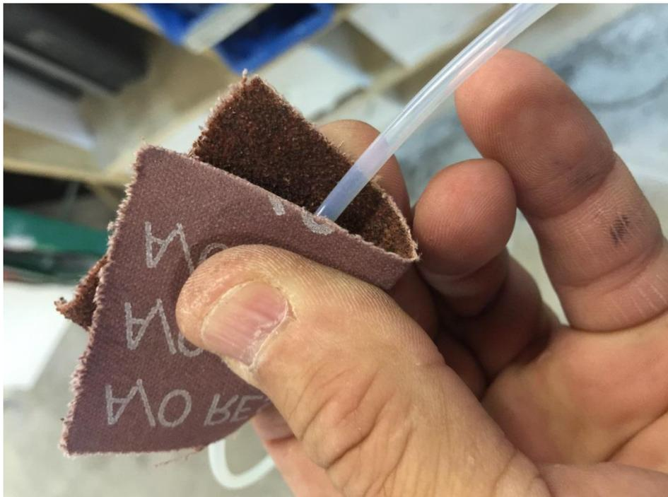
The easiest way to do this is by folding the sand paper and pulling the Teflon™™ through.
