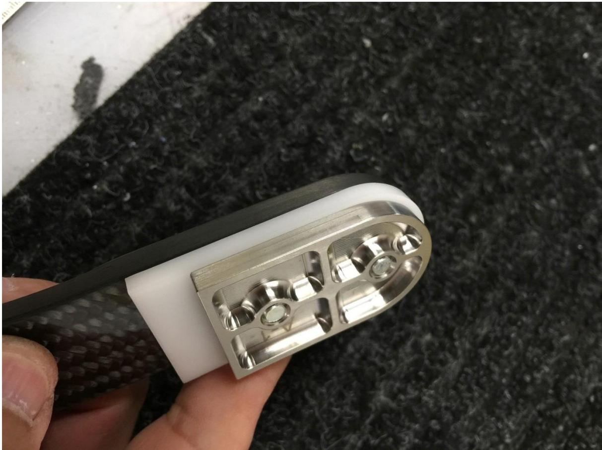
For fitting and attachment to the model the spring is assembled as shown. The white Delrin™ tooling must be included as this to maintain proper final alignment and space for the lamination materials.
