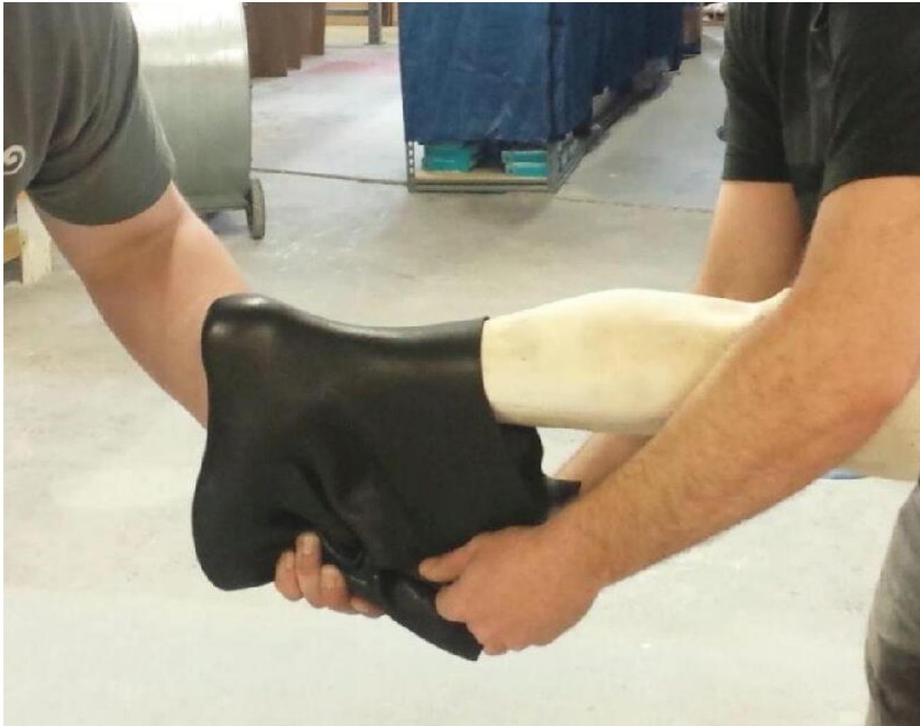
Using a 1/8" thick semi dense soft foam (Black Puff) pull a seamless boot for the entire foot section. Label this piece with patient information and set aside for finishing.
