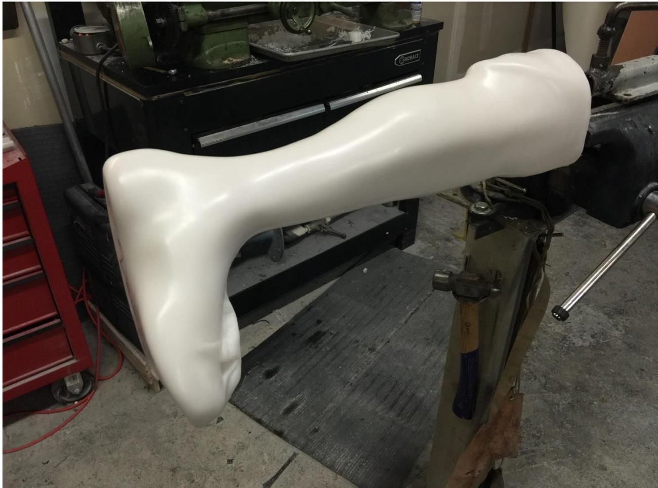
Using 1/8" thick polypropylene pull the entire model using the same technique you would use for a standard plastic AFO. Ensure there are no wrinkles or excessive stretch within the trim lines. This will serve as both a spacer for the plastic and foam liners as well as a releasable surface to laminate on.
