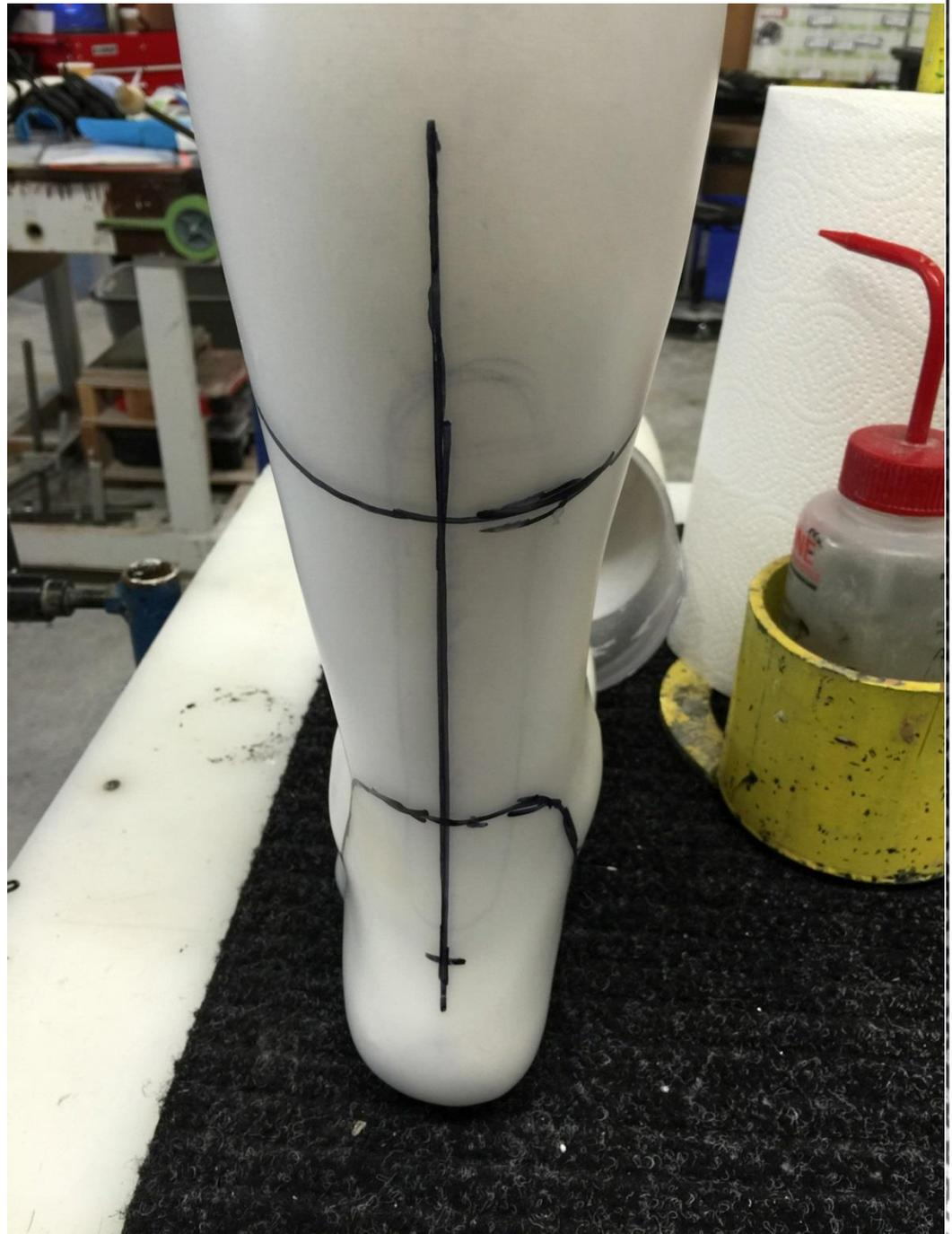
In a horizontal holder (vice) orient the model in a toe down position and set toe out. This will leave the line of progression in a vertical orientation.
