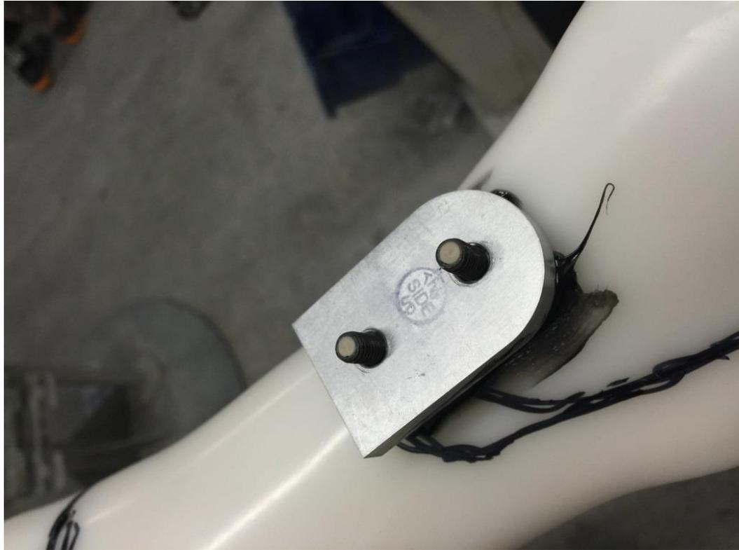
Remove attachment screws from the PDE assembly leaving only the anchor plates bonded to model. Insert the set screws from the anchor kit into the anchor plate until they bottom out. Be sure the set screws are treated with a mold release of some type and after the installation the Allen wrench holes are filled with clay.
